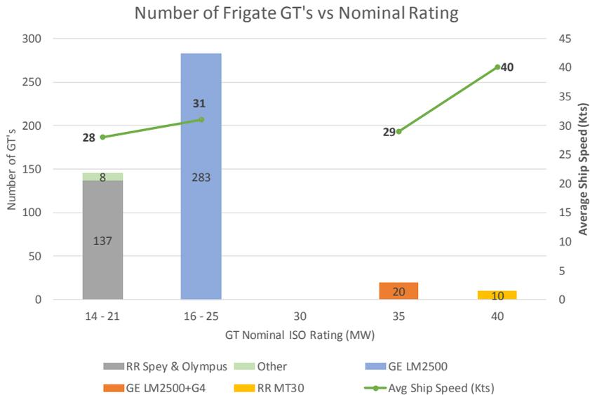
Figure 5: Gas Turbines on Active Commissioned Ships
