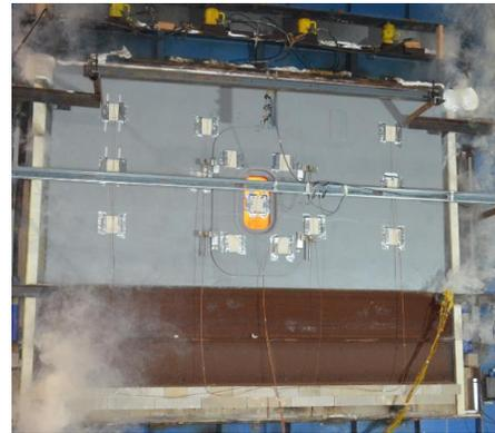
Figure 14: Composite Sidewall during Fire Resistance and Structural Integrity Validation Testing
