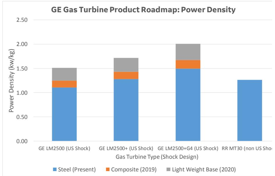
Figure 17: GE Gas Turbine and Module Power Density (kw/kg)
