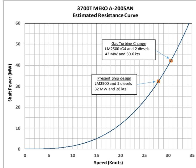
Figure 16: 3700T Estimated Ship Resistance Curve with LM2500+G4 Upgrade
