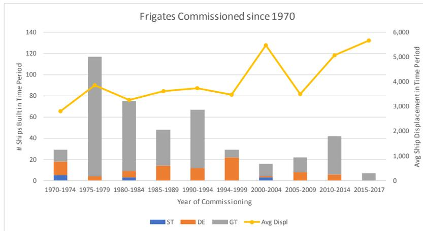
Figure 1: Frigate Propulsion Type and Displacement versus Time
