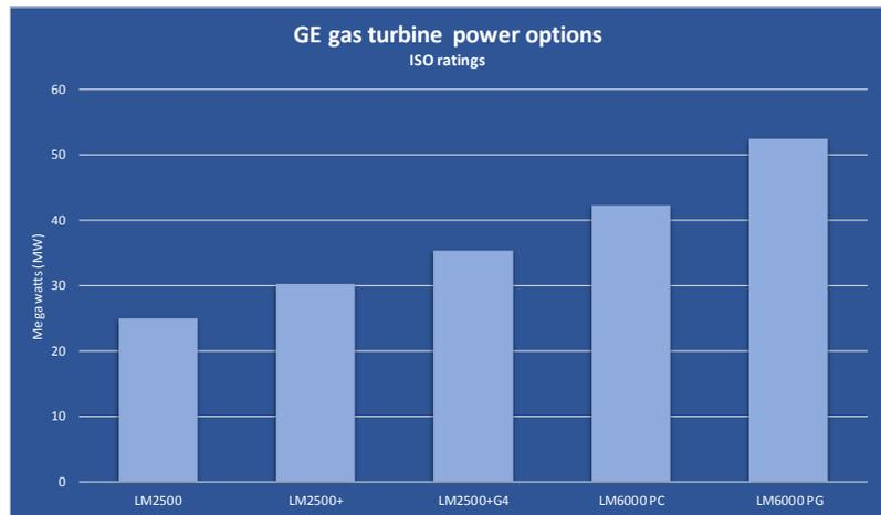
Figure 8: GE Marine Propulsion Gas Turbine Product Family
