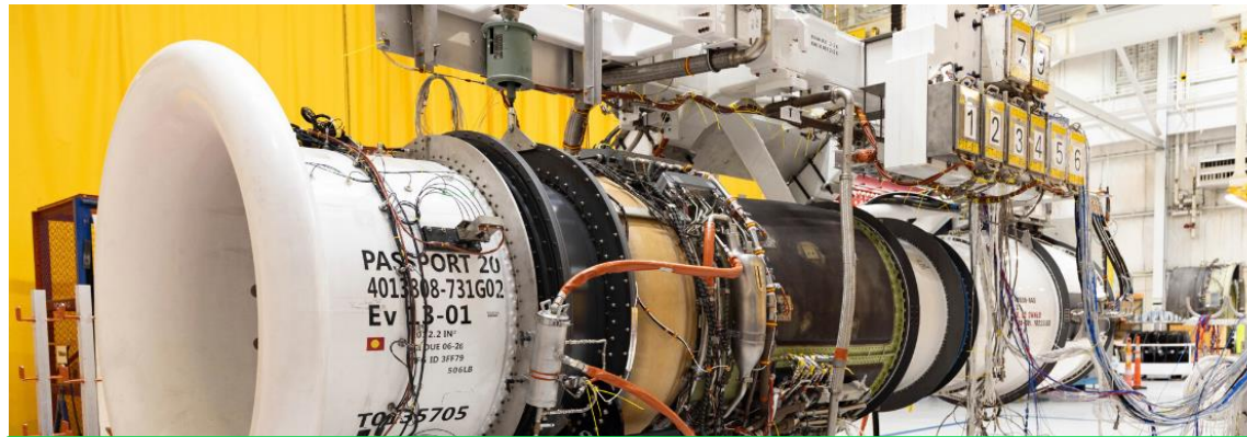
Ground test of first hybrid electric commercial engine demo to better understand controls and integration
