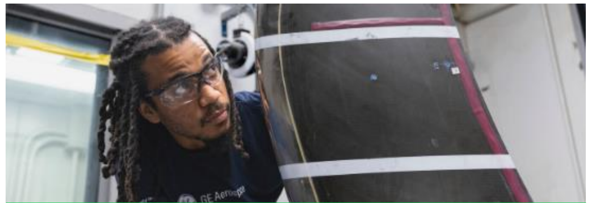
Testing full-size Open Fan blades and vanes ... building on composite expertise for lighter blade, leveraging Dowty Propeller experience for blade attachment
