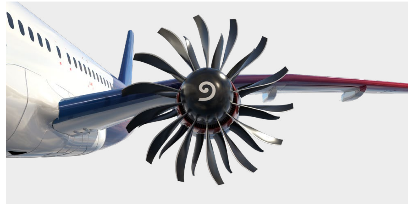
Rendering of the CFM RISE Open Fan engine architecture on wing.
