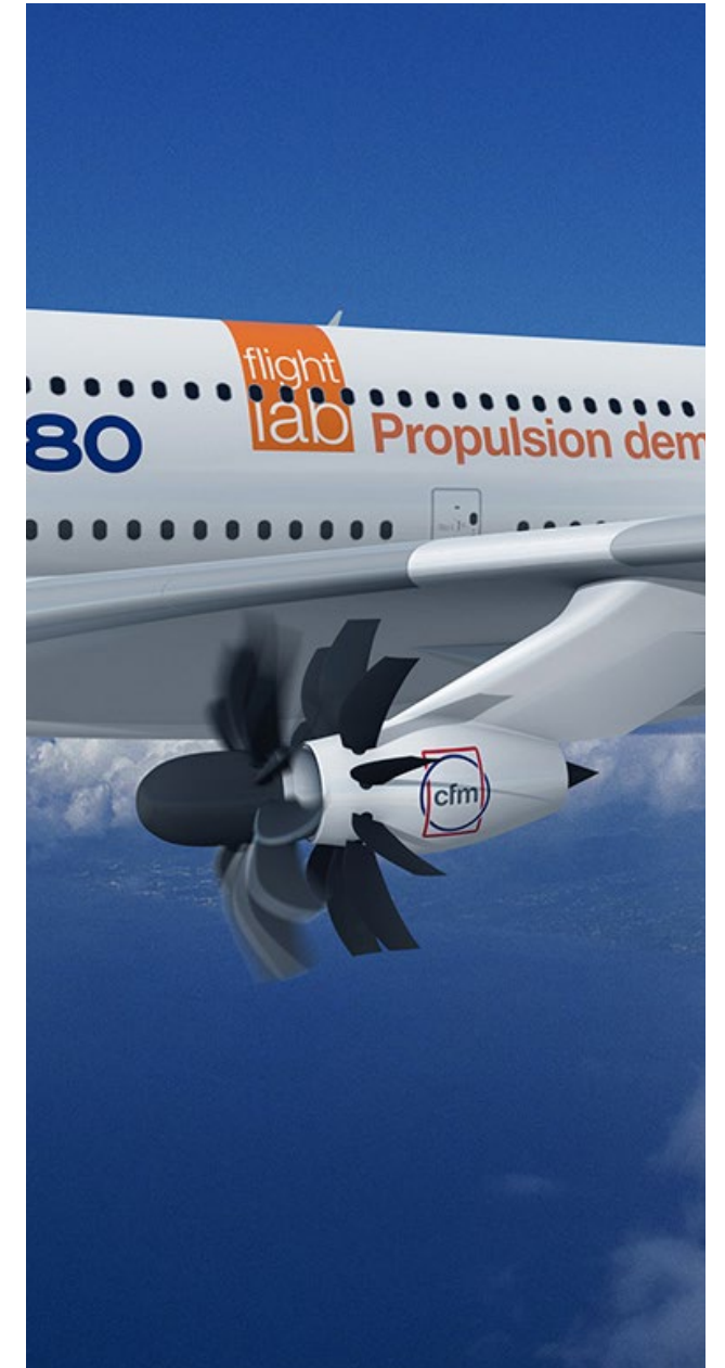
CFM International and Airbus plan to flight test Open Fan engine architecture this decade. Image credit: Airbus.
