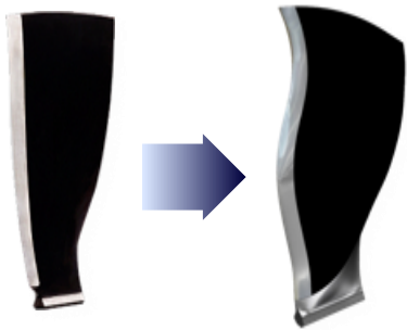
GE90-94B composite fan blade introduced 1995
